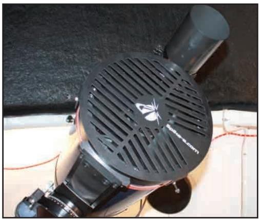
Image 3 - Always place your mask on your scope in the same orientation. The author aligns his mask so the logo is upright and the center column of aluminum is in line with the counterweight shaft.
